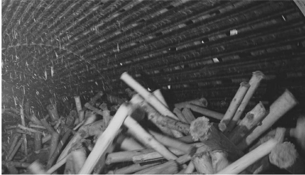
FIGURE 32.4 Bark removal from cut wood in a rotating debarking drum.
