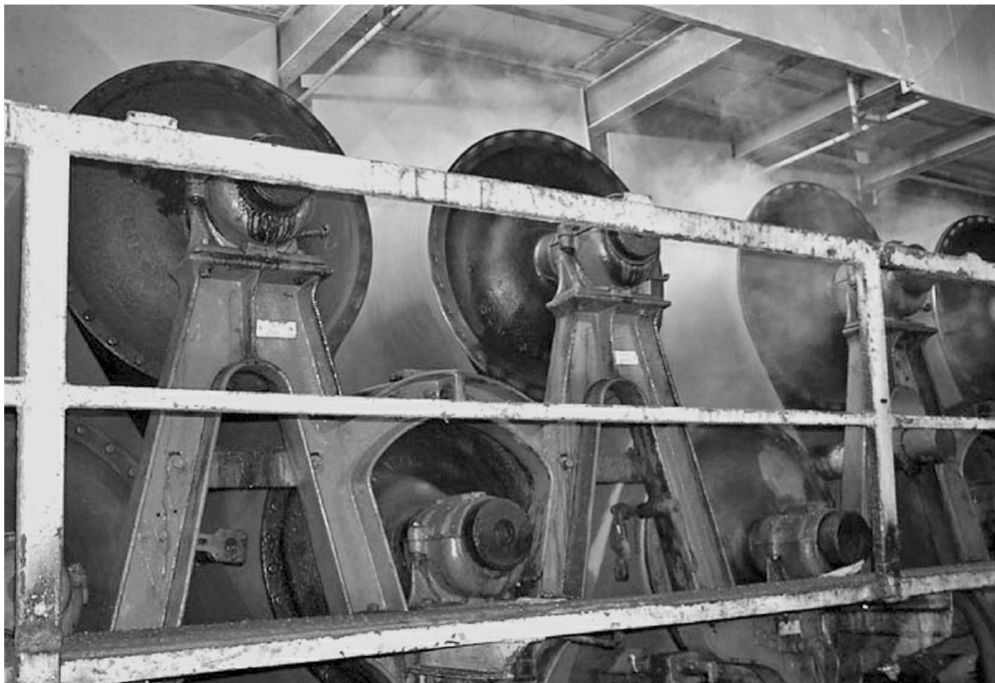
FIGURE 32.18 Steam heated dryers evaporating the remaining water.
