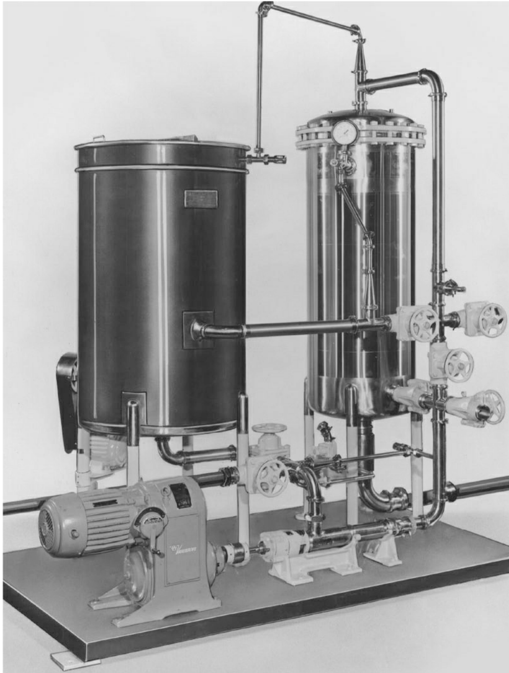
FIGURE 40.4 Typical filter installation in the food and beverage industry. Note the use of special stainless steel piping and fittings. ( Courtesy of Croll-Reynolds Engineering Company, Inc. )
