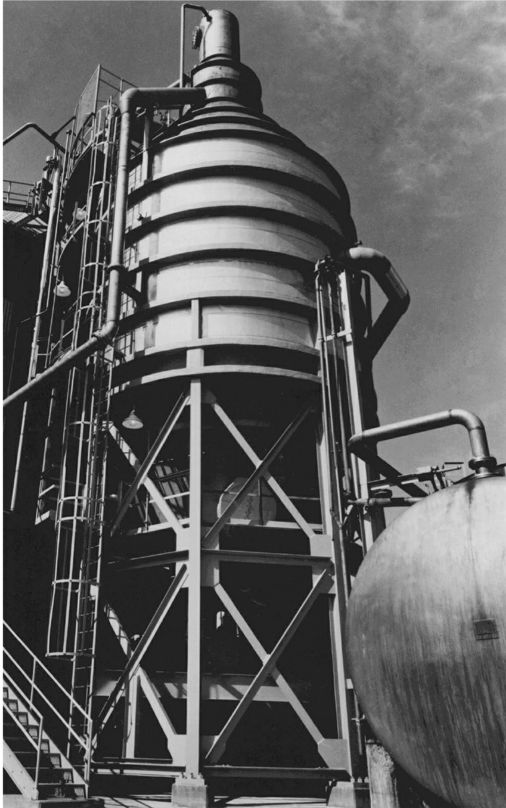
FIGURE 36.8 A large crystallizer producing ammonium sulfate. ( Courtesy of Whiting Corporation. )
